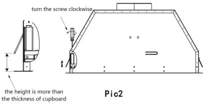
4. Put the hood into the cabinet, and then use screwdriver to turn the 4pcs buckle screws anticlockwise separately until the panel of hood fit to the cabinet horizontally and make sure the hood is secured.See pic3&4.
